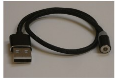
Photo 1: Magnetic Power Cable
