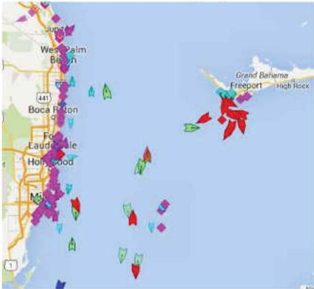
Vessels over 299GT (Gross Tonnage) are required to have an AIS transponder on board, which transmits their position, speed and course, among some other static information, such as vessel's name, dimensions and voyage details.
